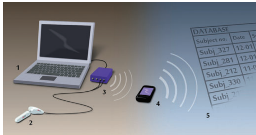
Figure 1 Schematic overview of the ambulatory measurement setting. (1) Generic laptop, (2) genital probe, (3) wireless sensor system, (4) handheld computer, and (5) secure central database. See text “Ambulatory laboratory” for detailed description.
